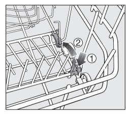
■ Press the yellow lever down ① and fold the spikes down ②.
